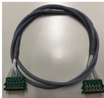
Figure 10: C-GEM HV On Detector Cables
